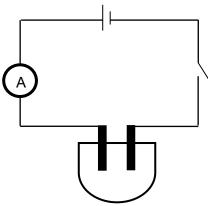
The anhydrous  $AgNO_3$  was added to 200 cm<sup>3</sup> distilled water spoon by spoon. The ammeter reading was recorded after each spoon was added. The results are shown in the table below.
