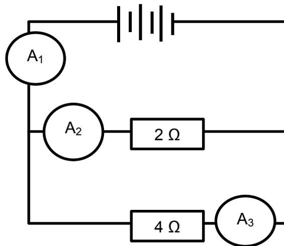
How will the readings on ammeters  $A_1$ ,  $A_2$  and  $A_3$  compare with each other?
