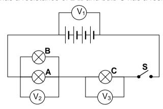
12.1 Calculate the effective resistance of bulbs **A** and **B**. (3)
